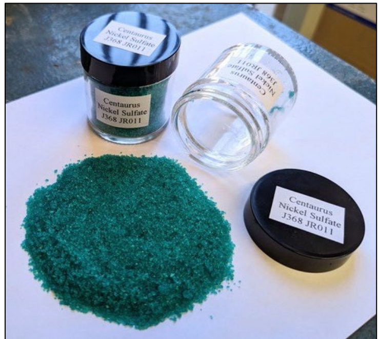
Figure 1: First nickel sulphate from Jaguar Pilot Plant Program.
