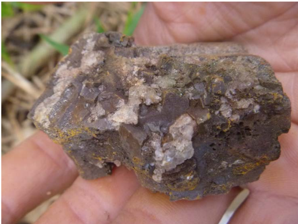
Figure 4 – Quartz vein with Limonite pseudomorphs after pyrite with boxworks (674377mE, 7851107mN).
