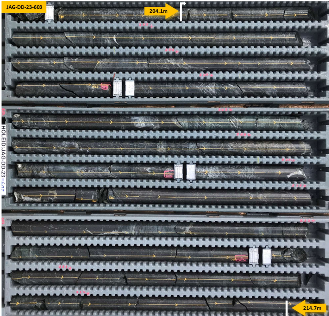
Figure 8 – The Twister Prospect: Core photo from drill hole JAG-DD-23-603; 204.1m to 214.7.0m down-hole: Stringer sulphides (dark metallic bronze) mineralisation associated with strong magnetite alteration (black).
