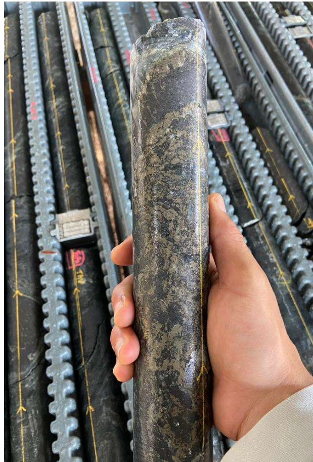
Figure 1 – Net-textured to semi-massive nickel sulphide mineralisation and magnetite alteration in JAG-DD-23-603 from 207.7m, intersected 100m down-dip from JAG-RC-23-191 which returned 11.0m at 1.06% Ni from 163.0m on cross-sections 478940mE.
