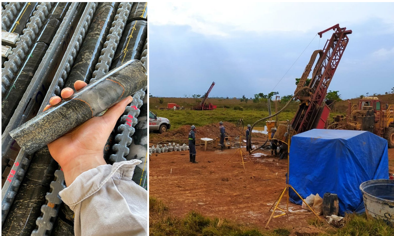
Figure 1 – Net-textured to semi-massive nickel sulphide mineralisation in the first diamond hole at the Tigre Prospect (left) and photo of diamond rig (background) drilling side-by-side with RC rig (foreground) at the Tigre Prospect.
