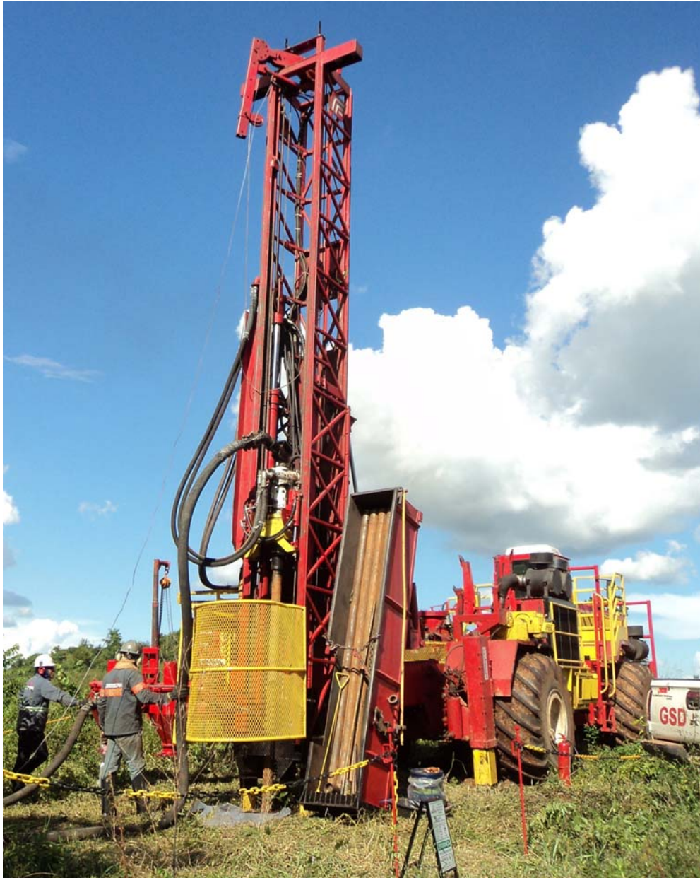
Figure 1 – Geosedna RC rig drilling on ITAP-RC-18-001, the first ever drill hole into the Itapitanga Nickel-Cobalt Project.
