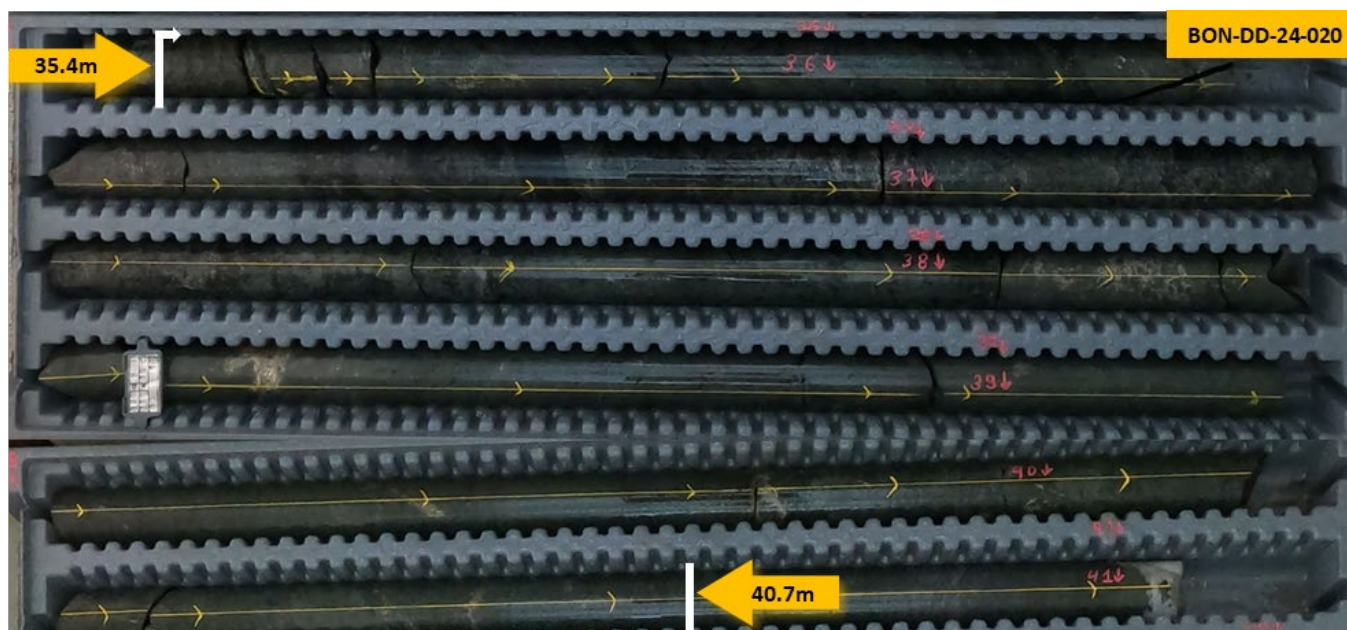
Figure 7 – The Nelore West Prospect: core photo from drill-hole BON-DD-24-020; 35.4 to 40.7m down-hole. See Table 2 for visual sulphide estimates. Stringer and semi-massive (dark metallic bronze) mineralisation with altered mafic host rock.
