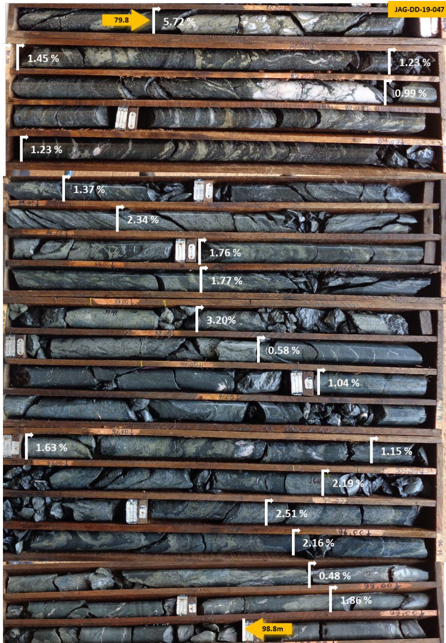
Figure 11 – Core photos from drill hole JAG-DD-20-047 (Jaguar Central); 79.8 to 98.8m: Stringer to semi-massive and local massive sulphides (metallic bronze/yellow colour) hosted in porphyritic dacite with local intense magnetite-chlorite-biotite alteration. Sulphides comprise pyrite, pentlandite, millerite, sphalerite and minor chalcopyrite - This interval returned 19.0m at 1.70% Ni, 0.13% Cu and 0.04% Co from 79.8m and is part of the broader interval of 67.3m at 1.20 % Ni, 0.08% Cu and 0.03% Co from 67.0m.
