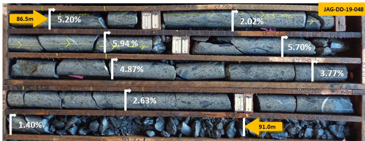
Figure 6 – Core photos from JAG-DD-20-048; 86.5 to 91.0m: Semi-massive and massive sulphides (metallic bronze/yellow colour) in granite with intense magnetite alteration (black). Sulphides comprise pyrite, pentlandite, millerite, sphalerite and chalcocite. This interval returned 4.5m at 3.66% Ni, 0.63% Cu and 0.17% Co from 86.5m.
