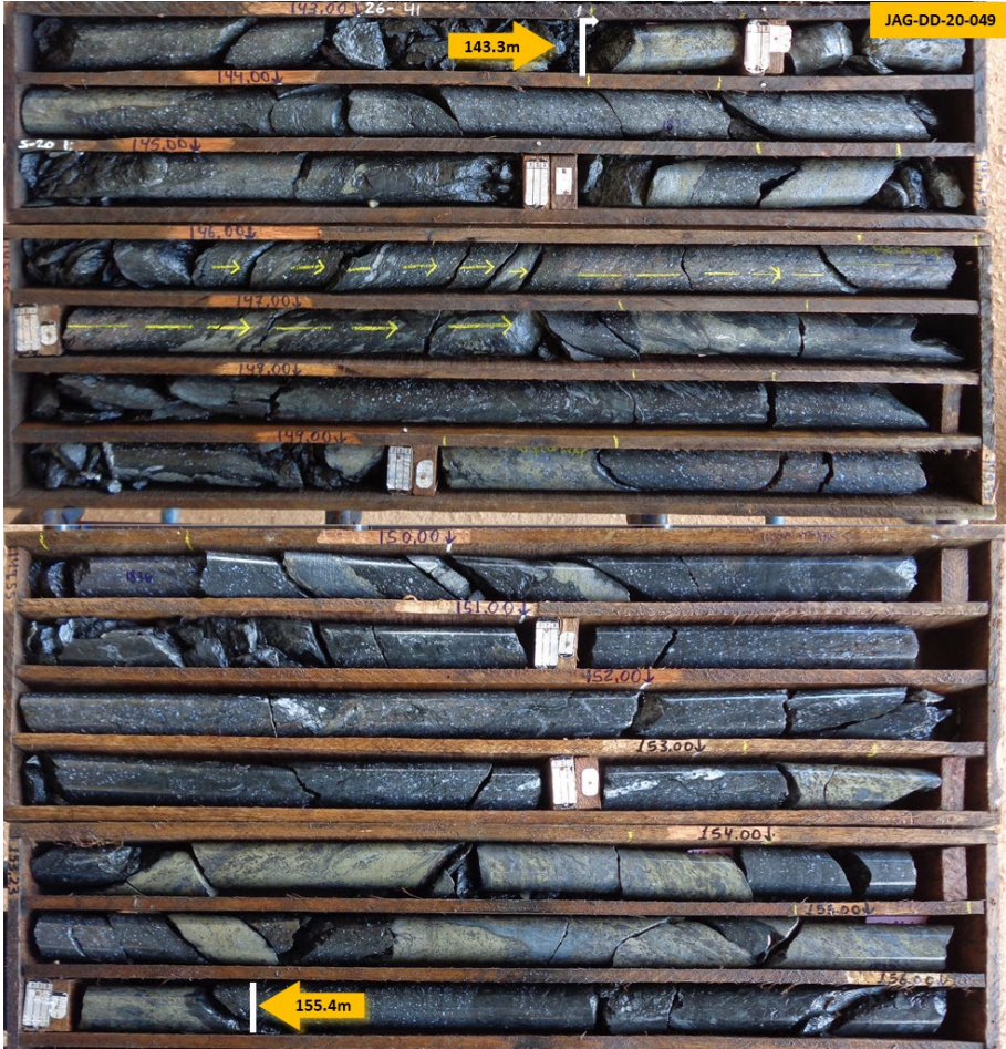
Figure 14 – Core photos from drill hole JAG-DD-20-049 (Jaguar Central); 143.3 to 155.4m: Stringer to semi-massive and massive sulphides (metallic bronze/yellow colour) hosted in porphyritic dacite with intense magnetite-biotite alteration. 5-20% sulphide content comprising pyrite, pentlandite, millerite, sphalerite and minor chalcopyrite - Assays pending.
