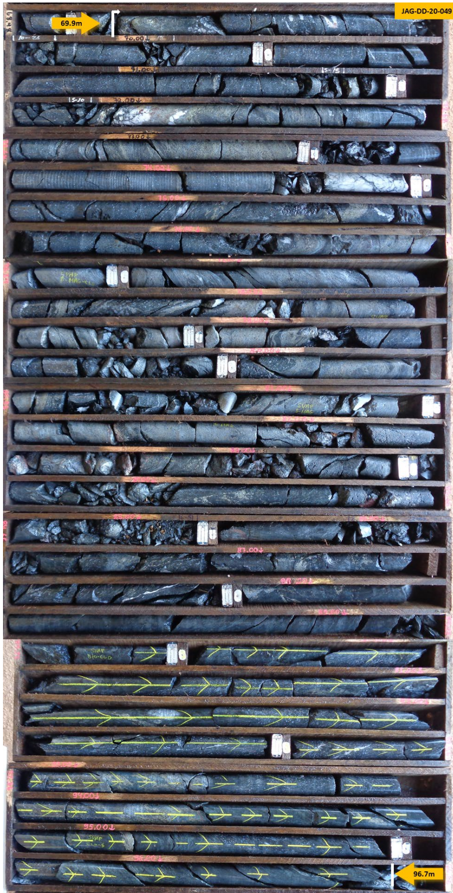
Figure 13 – Core photos from drill hole JAG-DD-20-049 (Jaguar Central); 69.9 to 96.7m: Stringer to semi-massive sulphides (metallic bronze/yellow colour) hosted in porphyritic dacite with local intense magnetite-chlorite-biotite alteration. 5-10% sulphide content comprising pyrite, pentlandite, millerite, sphalerite and minor chalcopyrite - Assays pending.
