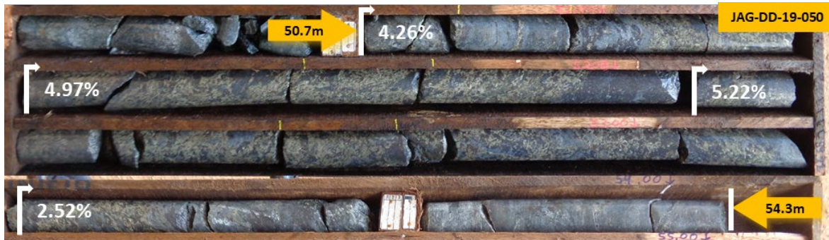
Figure 7 – Core photos from JAG-DD-20-050; 50.7 to 54.3m: Semi-massive and massive sulphides (metallic bronze/yellow colour) in granite with intense magnetite alteration (black). Sulphides comprise pyrite, pentlandite, millerite, sphalerite and chalcopyrite. This interval returned 3.6m at 4.24% Ni, 0.49% Cu and 0.16% Co from 50.7m.
