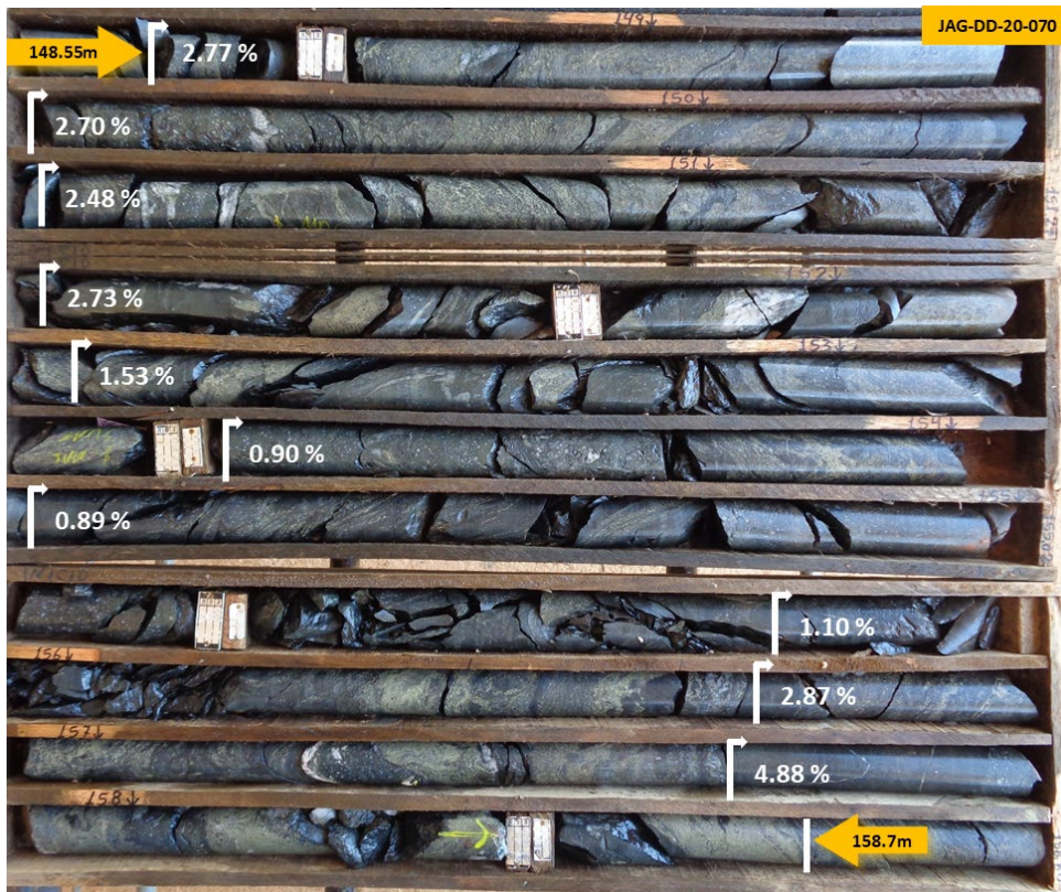
Figure 4 – Core photo from drill hole JAG-DD-20-070 (Jagaur Central); 148.55m to 158.7m down-hole: Stringer to semi-massive and massive sulphides (metallic bronze/yellow colour) with magnetite (black colour) mineralisation hosted in altered dacite. 10-20% sulphide content comprising pyrite, pentlandite, millerite, sphalerite and minor chalcocopyrite – this interval returned 10.2m at 2.22% Ni, 0.25% Cu and 0.04% Co.
