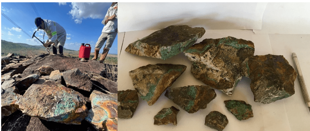
Figure 4 – The Boi Novo Project: Malachite and chalcopyrite identified in outcropping mafic and tonalitic rocks.
