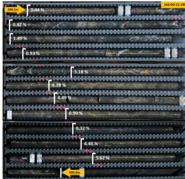
Figure 1 – Core photo from drill hole JAG-DD-21-190 (Onça Preta); 299.2m to 309.9m down-hole: Disseminated, stringer to semi-massive sulphides (metallic bronze/yellow colour) with intense magnetite (black colour) mineralisation hosted in basement gneiss.
