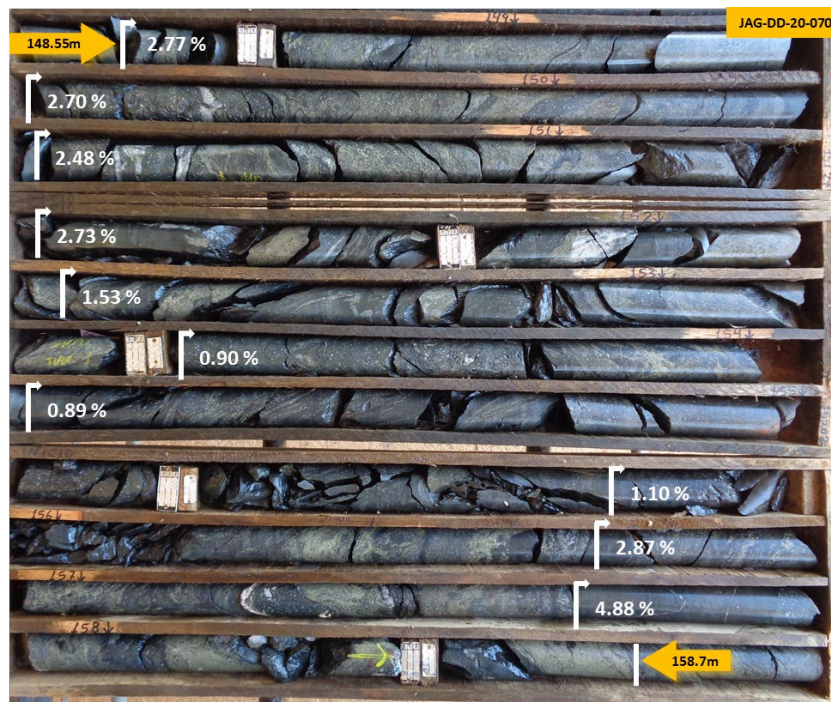
Figure 4 – Core photo from drill hole JAG-DD-20-070 (Jaguar Central), 148.55m to 158.7m down-hole: Stringer to semi-massive and massive sulphides (metallic bronze/yellow colour) with magnetite (black colour) mineralisation hosted in altered dacite. 5-10% sulphide content comprising pyrite, pentlandite, millerite, sphalerite and minor chalcopyrite – This interval returned 10.2m at 2.22% Ni, 0.25% Cu and 0.04% Co.
