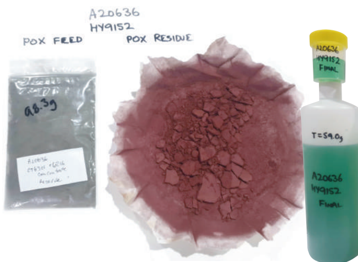
Figure 15 - Jaguar Nickel Sulphide Pressure Oxidation images. The POx residue material would be sent to tailings. The green POx nickel solution will be crystallised to produce a nickel sulphate product
