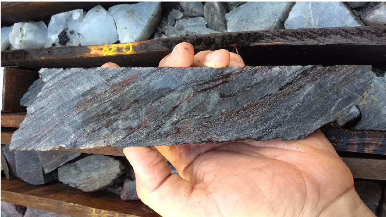
Figure 3 – SRM-DD-17-002 intersected a hydrothermal breccia with silica and muscovite alteration plus sulphides (6m at 0.7g/t Au from 84m, including 2m at 1.35 g/t Au; photo: 84.3m – 1.8g/t Au)
