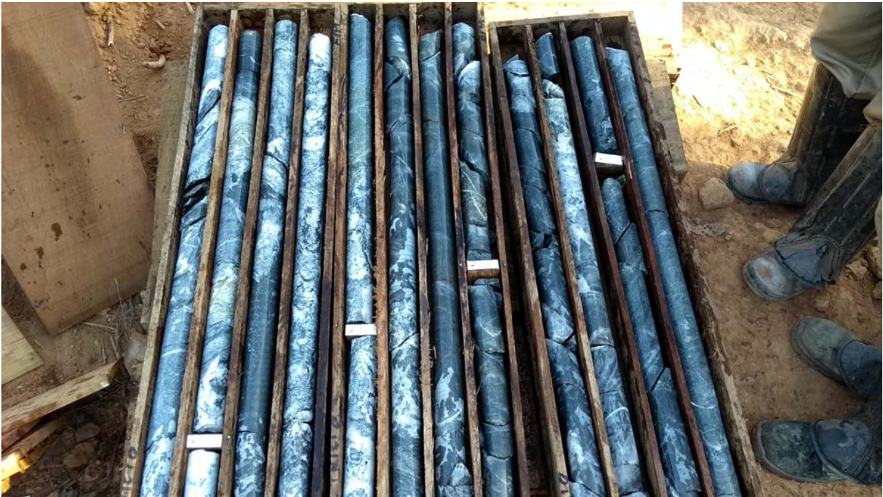
Figure 2 – SRM-DD-17-001 from 242.3m brecciated quartz veining, intense silica alteration and localised carbonate alteration plus sulphides (20.3m at 0.05g/t Au from 241.7m).
