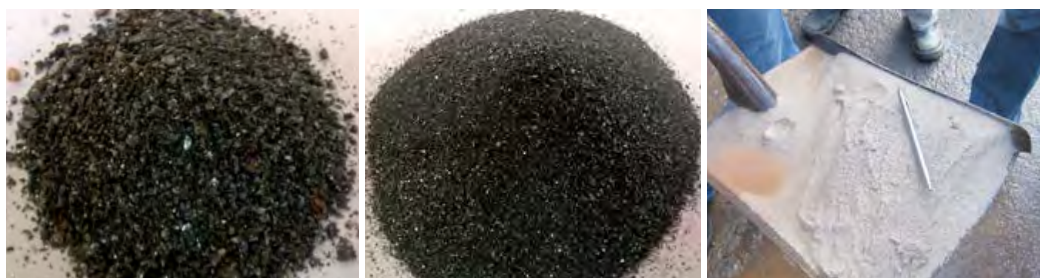
Figure 6 - (Left to Right) Jig Concentrate, WHIMS Cleaner Concentrate, Tails from WHIMS Cleaner Process
